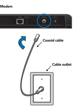
Connect the coaxial cable emerging from your cable outlet to the CABLE port located on the back of the modem.
